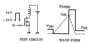
$$\begin{aligned} &R_G = 25~\Omega \\ &V_{DD} = 90~V,~L = 4.41~mH \end{aligned} \qquad E_{AS} = \frac{1}{2} \cdot L \cdot I^2 \cdot \left( \frac{B_{VDSS}}{B_{VDSS} - V_{DD}} \right) \end{aligned}$$
