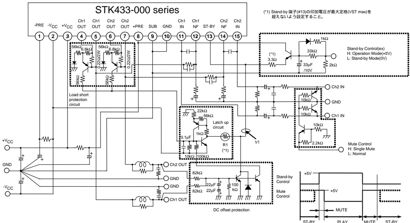
(\*1) R1 is changed depending on the power-supply voltage (-VCC).
